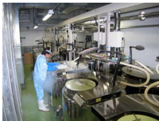
Cryopreserved embryos and sperm are stored in the liquid nitrogen tanks for many years.
