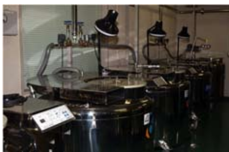
Liquid nitrogen tanks
