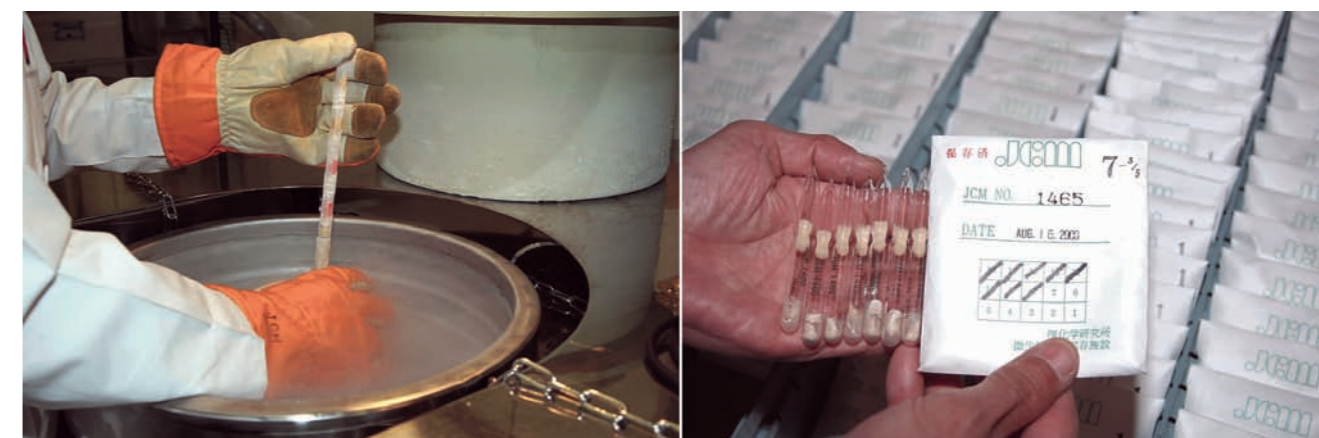
左：液体窒素下での微生物株の保存。右：提供用の微生物株の凍結乾燥標品 (図1) Left : preservation of microbial cultures in liquid nitrogen tank. Right : Ampoules of freeze-dried microbial cultures used for distributions. (Fig.1)
